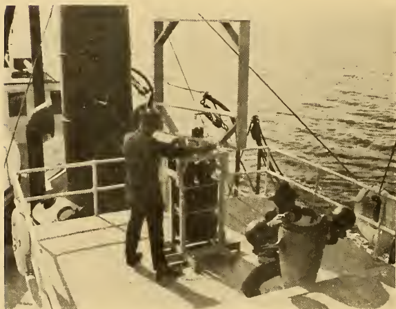
FIG. 32.—Experimental type of direction finder on lighthouse tender "Arbutus"
