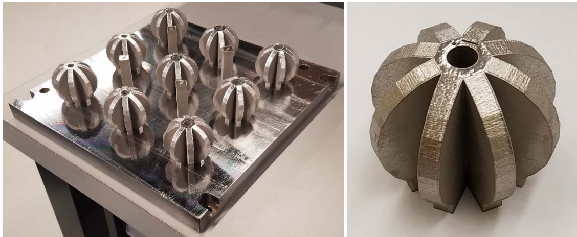
Fig. 5. Image of the build (left) and one of the artifacts after it was removed from the build plate (right).
