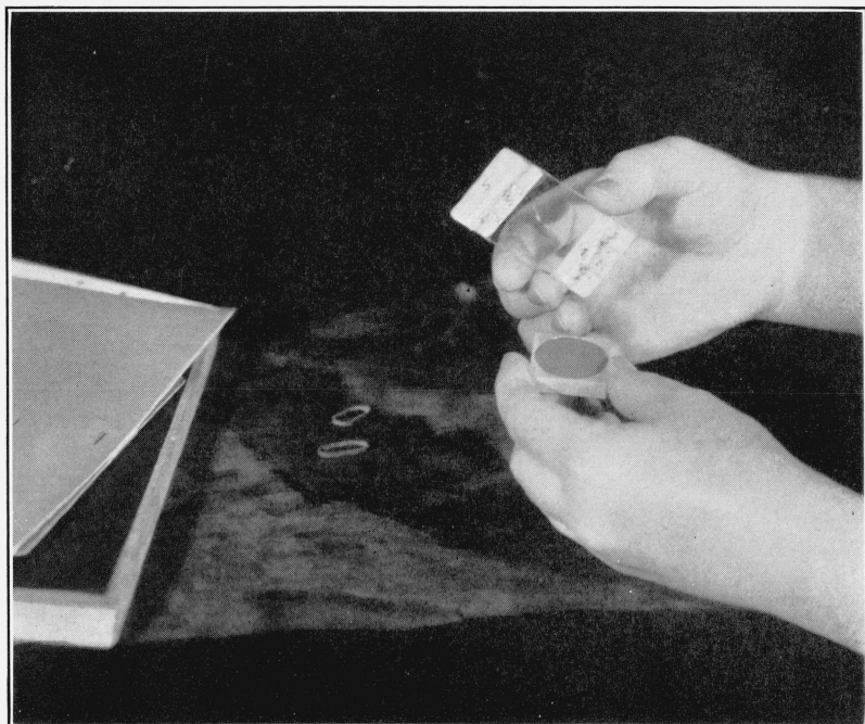
FIGURE 3.— Preparation of an opaque-powder sample for comparison with the Munsell color standards.
