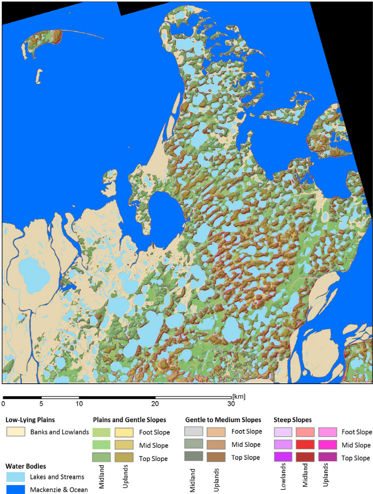
Figure 4.78: Landform classification of Northern Mackenzie Delta based on a TPI scale of 1500 m and elevation and slope. Source: Own Figure.
