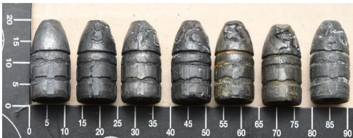
Figure 5.11: Combined .45 Colt calibre LRN bullets recovered from the Muscle of Human 2, with increasing exposure time (left to right).
