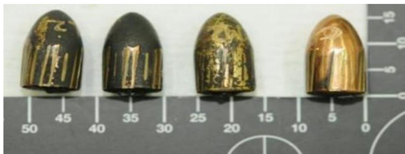
Figure 4.5: 9mm Parabellum calibre bullets recovered from Pig, indicating the corrosion products (left to right):
