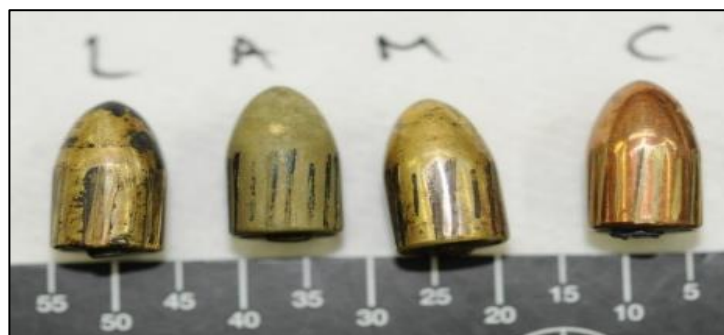
Figure 4.8: 9mm Parabellum calibre bullets recovered from Pig 1, indicating the following colours (left to right): Bright gold with some black scaling (labelled L), dull gold (labelled A), bright gold (labelled M) and untarnished copper, the control bullet (labelled C)
