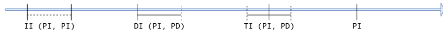
Figure 5.8: Timeline of all four absolute temporal expressions expressible using only the Time language. The indicated involved concepts are named after the initials of concepts shown in Figure 5.6 on page 92. Normal lines indicate properties defined by the user, dashed lines are the resulting temporal boundaries.
