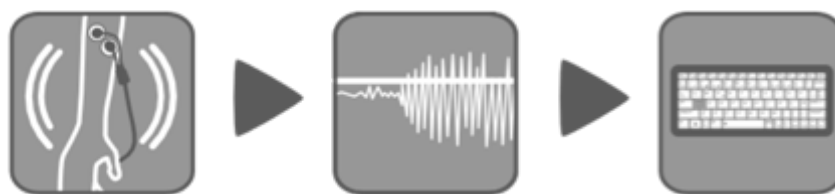
Figure 30 - Block diagram of the proposed system: (1) Data acquisition - user activates the sensor generating input signals; (2) Signal processing - input signal is sent via Bluetooth to the computer and processed to generate commands; (3) Switch-based control - when an event is detected, the system sends a command to an assistive communication software (e.g. a virtual keyboard)
