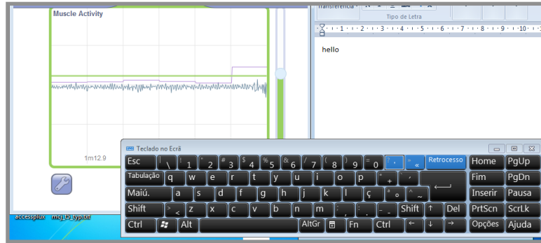
Figure 32 - Example of the developed platform, controlling an onscreen keyboard to perform a writing task in a ©WordPad (from Microsoft) document. In this example, when detecting a control signal from EMG generated by the user, the key “Enter” is sent by the platform to the application of onscreen keyboard. This command performs a selection using the scanning method.
