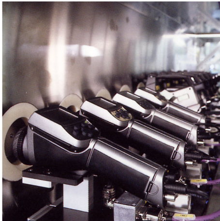
Figure 30.5 LEFT: Testing of infrared cameras in the climatic chamber; RIGHT: Robot used for camera testing and calibration
