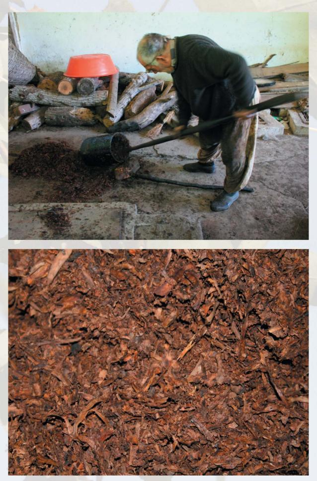
The shavings boiled are taken from the boiler via spoons, compressed via presses and sweet gum oil is degreased and collected in concrete pools.
