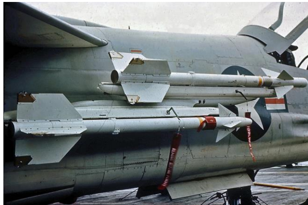
Figure 3 AIM-9C and D Sidewinders on an F-8E Source: US Navy
