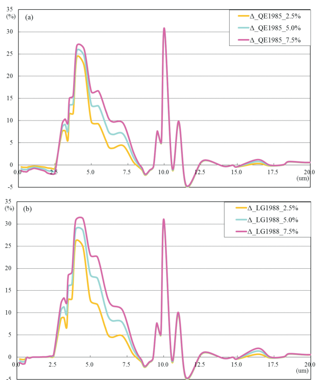
Figure 6. The difference \Delta\omega_0 between the single-scattering albedo (SSA) of pure illite and the single-scattering albedo of mixtures with different contents and refractive indices of hematite. (a) Complex refractive index of hematite from Query (1985), (b) complex refractive index of hematite from Longtin (1988).
