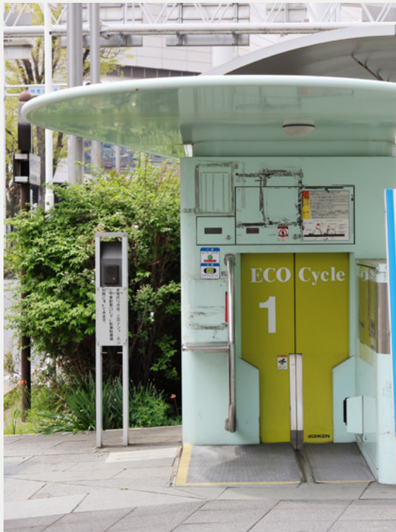
Automated cycle storage that parks and retrieves the user's cycle
