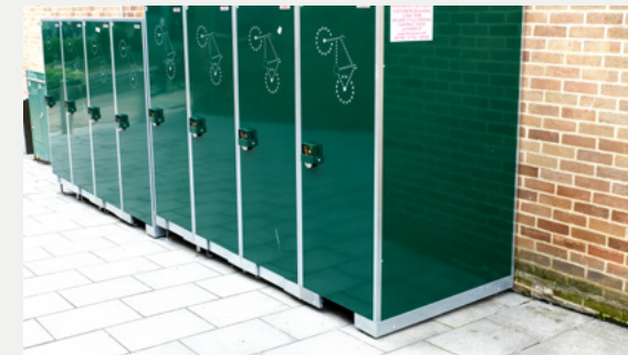
Vertical cycle lockers. Users have to be able to lift their cycles high, so these lockers may only be suitable for strong users or those with lightweight cycles
