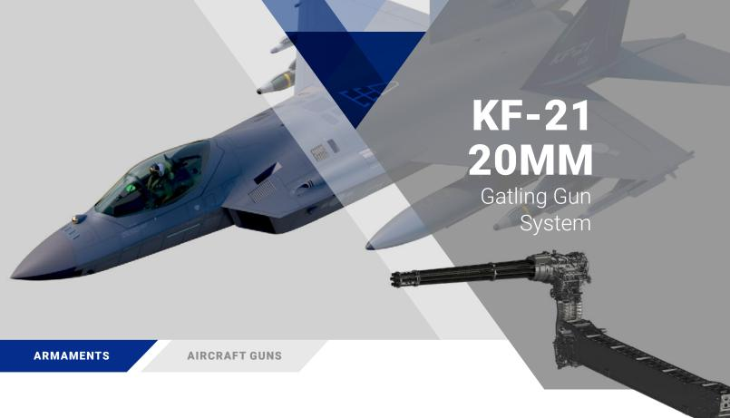
The KF-21 fighter is armed with the M61A2 20mm Gatling gun system produced by General Dynamics Ordnance and Tactical Systems. The fixed-forward internal gun system provides maximum firing rate performance.
