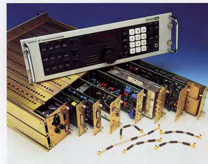
TERMA ("Dansk Radio") has also supplied the antenna tuners (TU 4015), synthesizers (SE 4010) and the HF-receivers (RX 4010) (shown above) for the THETIS-Class.
