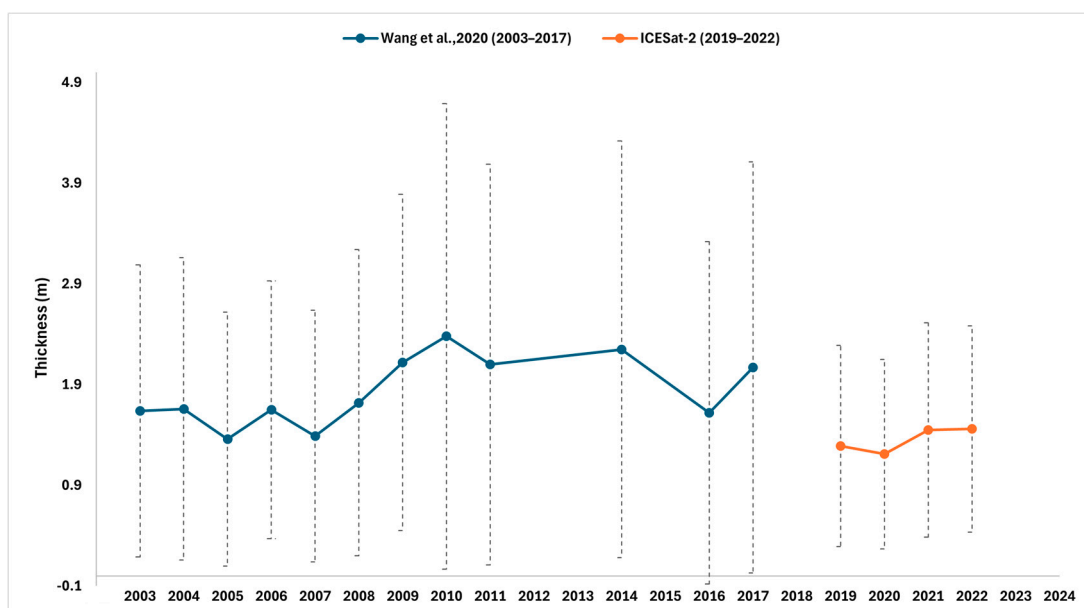
Figure 7. Comparison of ICESat and IceBridge mean thickness results in blue from [7] using the same method, with ICESat-2 results from this study in orange.
