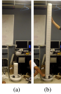
Fig. 1. The 57mm diameter Spiral Zipper starting to extend (a) and fully extended (b) [5].
