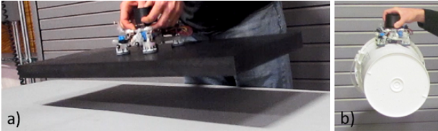
Fig. 10. Gripper grasping a) 15 kg slab of polycarbonate and b) 1.1 kg plastic bucket ( r = 13.8 cm at center).
