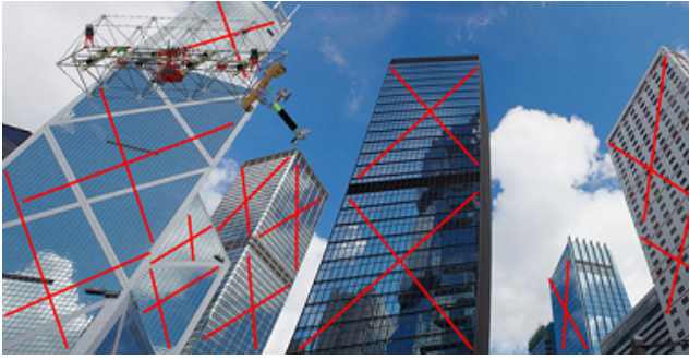
Fig. 1. Urban settings are rife with featureless surfaces such as glass and metal that could potentially be used as lateral grasp locations for a suction-based gripper, enabling the leveraging of large environmental forces.
