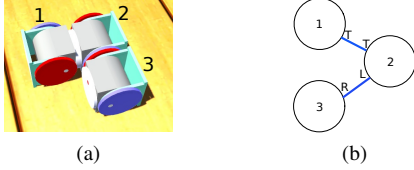
Fig. 3. (a) A three-module configuration and (b) its graph.
