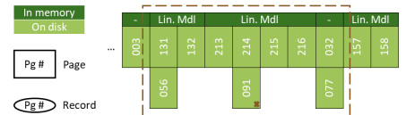
(a) Page 091 - the overflow for 214 - is full, causing reorganization. Phase I detects more segments with reorganization potential.
