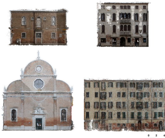
Figure 4. Automatically produced orthophotos of four buildings from a point-cloud obtained by street-level photogrammetry of the Campo Santa Margherita
