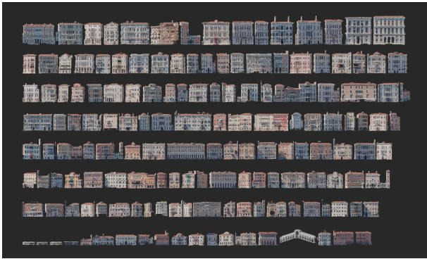
Figure 3. Orthophotos of 156 facades on the Canal Grande obtained following the automatic division of a city-scale photogrammetric model.
