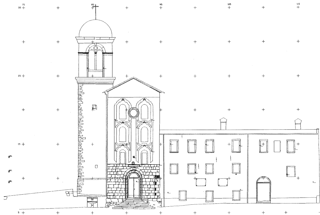
Figure 5 - The plotting of views of the exterior with the Wild Elcovision system.
