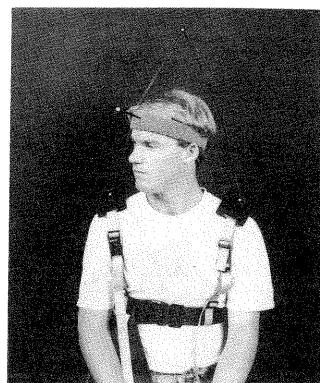
A normal Subject being recorded during axial rotation. Note: The targetted harness allows for shoulder movements to be mathematically isolated from head movements.
