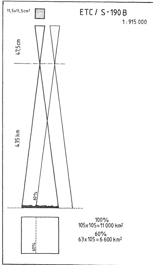
**Figure 1:** Disposition of camera during the S-190-B Earth Terrain Camera Experiment. Further explanation see text.
