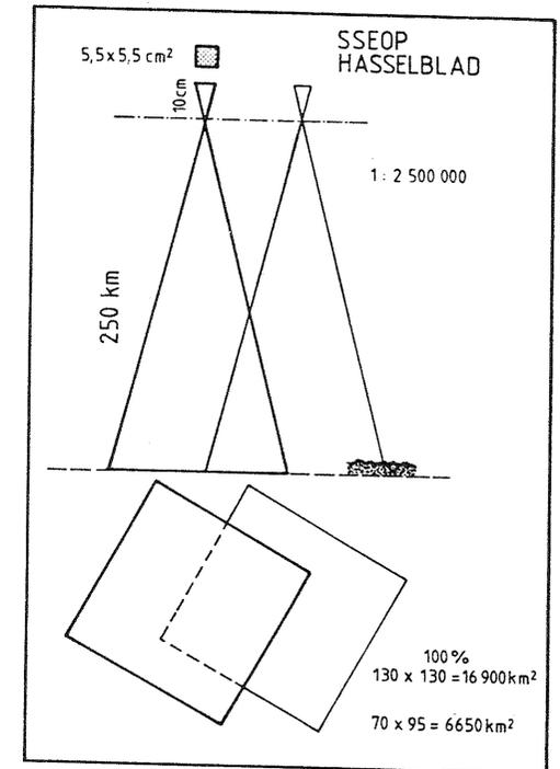
**Figure 4:** Disposition of camera for the data take of image pair 2708-2709 of orbit 58 of STS 9 Mission (SSEOP).
