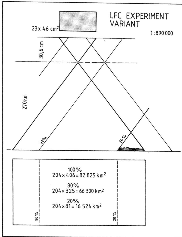
**Figure 3:** Representative disposition of camera during the Space Shuttle Large Format Camera Experiment. Further explanation see text.
