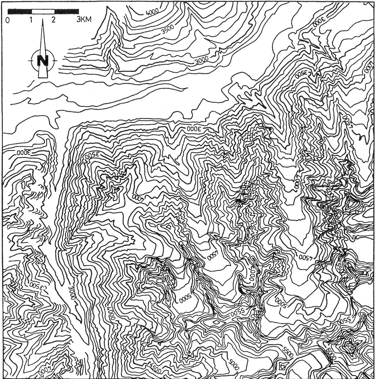
**Figure 6:** Contour line map of the Wark-Koh-e-Keshnikhan area in NE Afghanistan / Hindu Kush, based on LFC photography. Original restitution scale 1 : 100 000.
