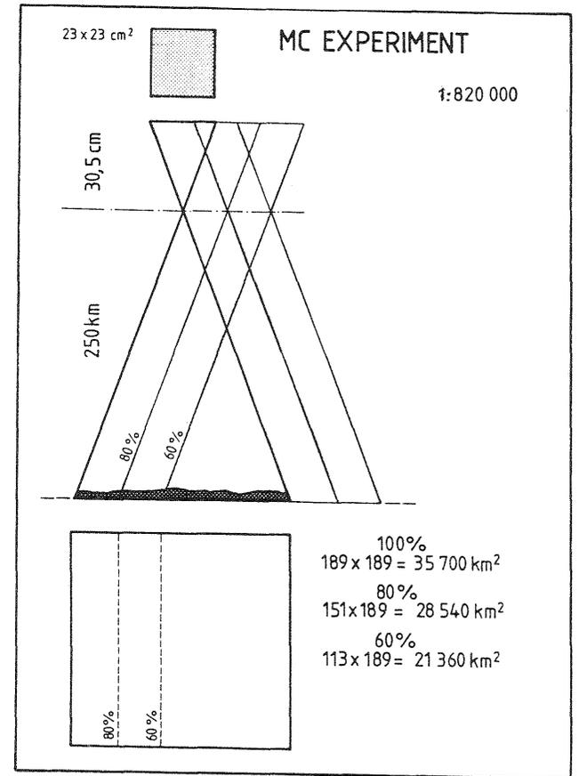
**Figure 2:** Disposition of camera during the Spacelab Metric Camera Experiment. Further explanation see text.
